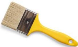
Before use, flick the bristles back and forth to remove dust. Make sure you remove excess liquid before painting. Fill the brush by dipping in up to half the length of the bristles. Tap it gently against the side of the can: don't wipe the brush hard against the lip. The bristles should flex only slightly as you brush – don't over press – let the paint flow from the brush.
